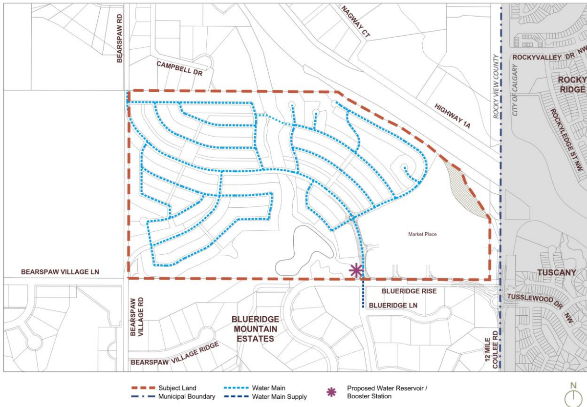
Figure 6: Internal Water Servicing Plan
