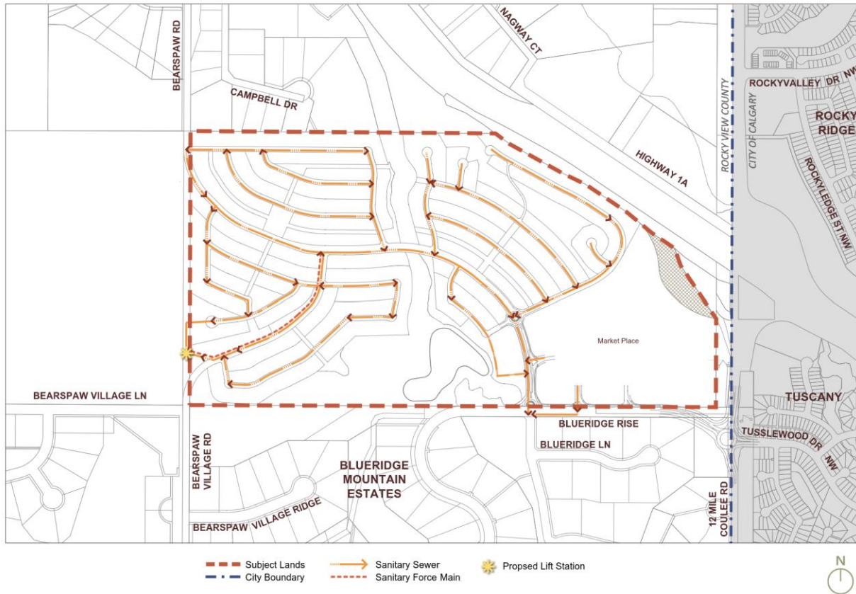
Figure 2: Internal Wastewater Servicing Plan
